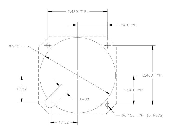
FIGURE 3-2 CUTOUT DIMENSIONS FOR PANEL MOUNTING
